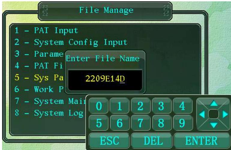
Save the Output of System Parameters being used in the system internal memory to USB flash disc.
