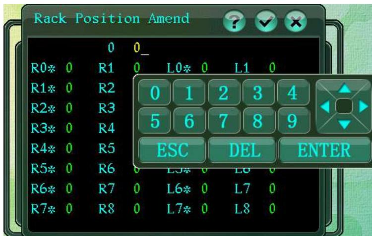
Rocking amendment is the system corrections for the difference between the positions of front and back needle plates.
