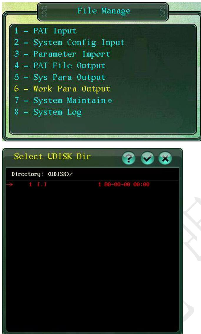
Save the Output of Operating Parameters of the pattern being used to the USB flash disk so that you can input them to the patterns that share the same settings.
