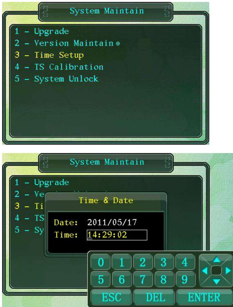
While installing and debugging a new machine, please first set the accurate system date and time.
