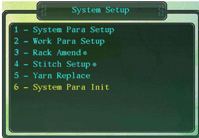
Reset system parameters to be the factory default. If the system parameters have been saved on the system parameter setting interface (by Key F2), the saved system parameters will be called automatically.
