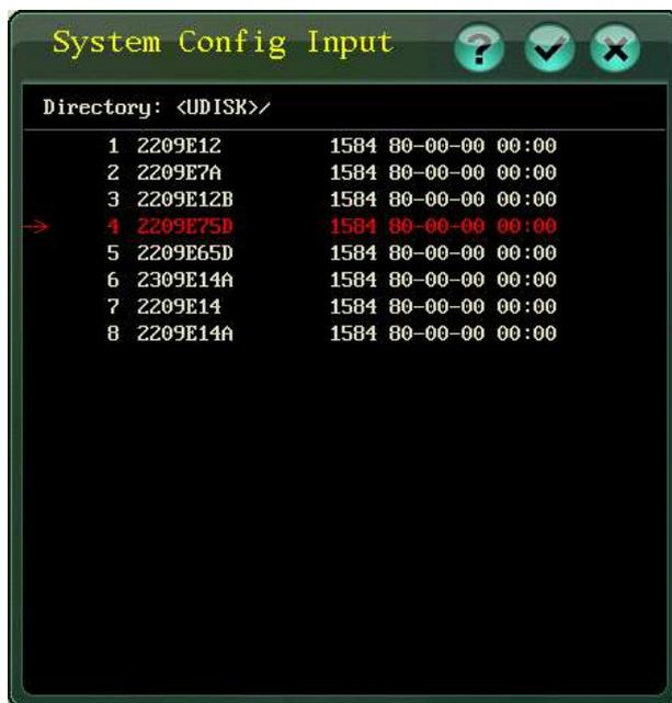
Save the Input System Parameters in the USB flash disk to current system internal memory
