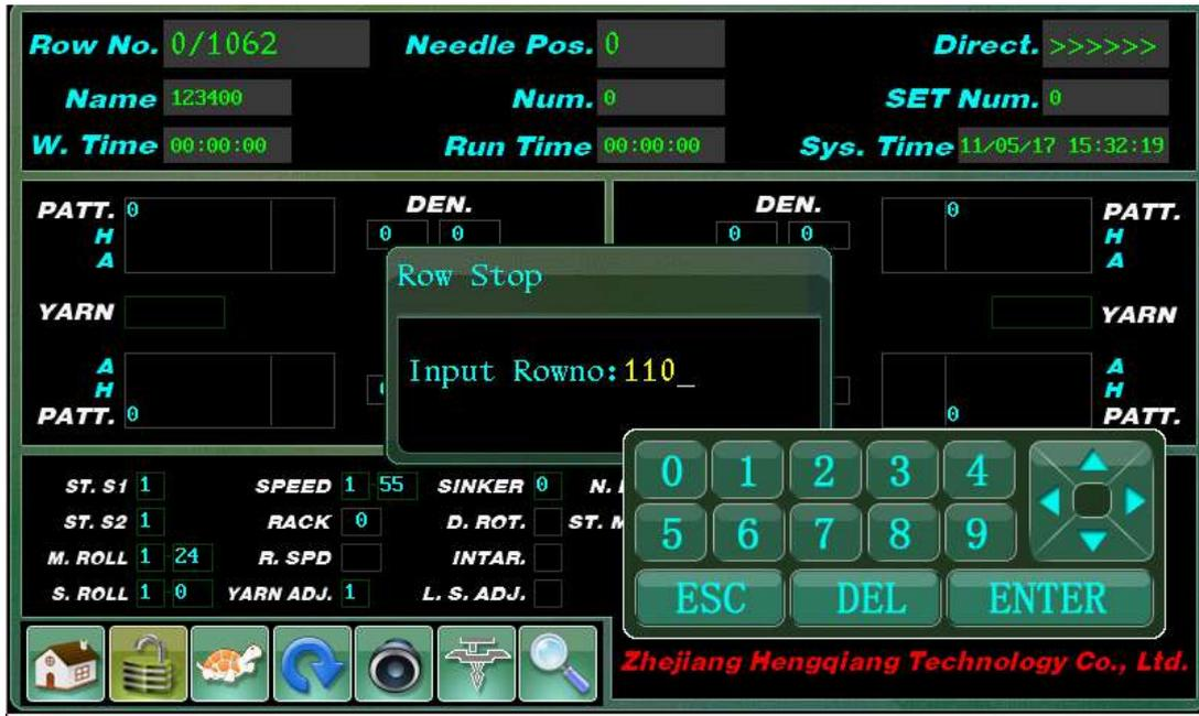
Keystroke: enter number of required stopping row and press Enter to complete.
