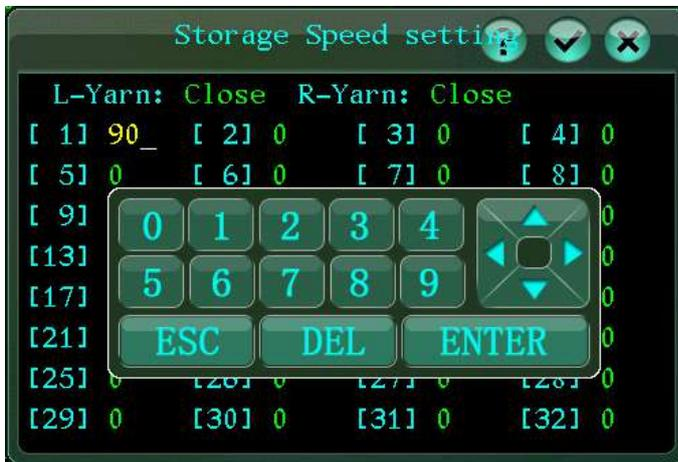
Keystroke: press “↑” “↓” “←” and “→” to the sections to be set. The font of fingers where the cursor stops is in red. Press Enter to modify, at the moment, the set values are of yellow font with white subscript. Input fingers and then press Enter key to complete.
